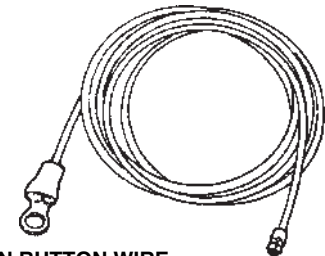
HORN BUTTON WIRE GOES FROM STEERING WHEEL DOWN COLUMN AND CONNECTS TO HEADLIGHT HARNESS. 1940 PASSENGER 01A-3671 EACH
