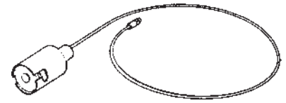
DASHLIGHT SOCKET WIRING CONNECTS TO DASH WIRING HARNESS
